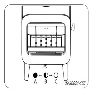
The primary air inlet regulates the air under the grate (1).
