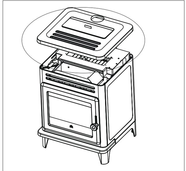
4. Undo the two screws on each side on the brackets underneath the top
